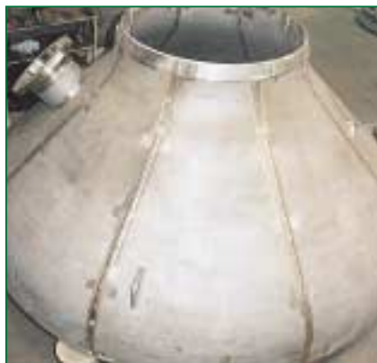
ANTONIUS Vesselheads built this 4.6 m-diameter, 60 mm-thick stainless steel toricone for Dow Chemical
